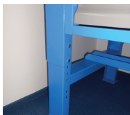
One of the main advantages of the new work benches are the height-adjustable legs.
